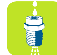
FLUSH nozzle with water to extract debris.
