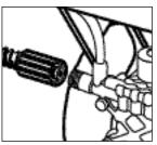
Step 6 Disconnect the high pressure hose from the high pressure outlet.
