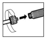
Step 3 Attach the wand to the spray gun.
