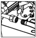
Step 7 Connect the garden hose to unit's water inlet.
