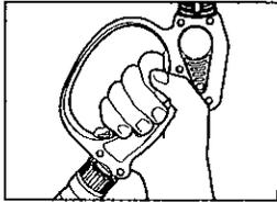
**Step 5** Press trigger to release water pressure.
