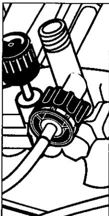
**Step 2** Adjust the dosage control at the beginning of the detergent tube for light (1), or maximum (6) detergent coverage.
