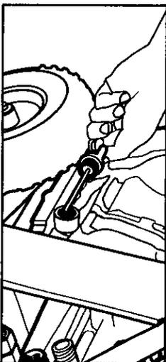
**Step 1** Check oil level. Oil level should be level with the bottom of the oil filler neck. Be sure the machine is level when checking the oil level. (Refer to the engine's operating manual for seasonal grades.) We recommend that the oil be changed after the first 5 hours of use, then once every 50 hours.
