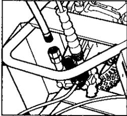
**Step 6** Disconnect garden hose from water inlet on the unit.
