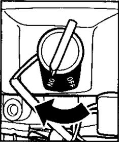
**Step 7** Turn the engine switch to the "ON" position.
