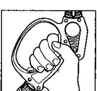
**Step 3** Press trigger to release water pressure.
