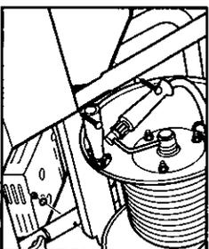
**Step 11** Attach the reel to the handle. Align holes, insert bolts, and tighten with nuts.
