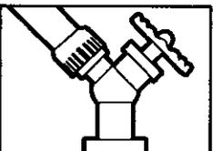
**Step 3** Connect garden hose to the cold water source and turn water on completely. Never use hot water.
