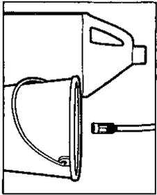
**Step 1** Remove detergent suction tube from container and insert into one gallon of fresh water. Siphon water at low pressure for one minute.
