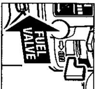
**Step 2** Slide fuel valve to the off position.
