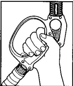
**Step 4** Trigger the gun to eliminate trapped air, wait for a steady flow of water to emerge from the spray nozzle.
