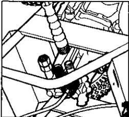
**Step 7** Disconnect high pressure hose from high pressure outlet.
