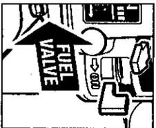
**Step 3** Slide fuel valve to the off position.
