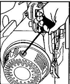
**Step 8** Pull the starter handle. If the engine fails to start after 3 pulls, squeeze the trigger gun to release pressure, and repeat step. After the engine is warm and running smoothly, slide the choke lever to the right (open) and throttle to the left (fast).
