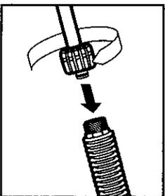
**Step 4** Attach the wand to the spray gun.
