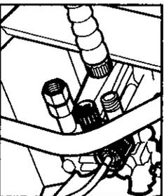
**Step 8** Connect the high pressure hose to the unit's high pressure outlet.
