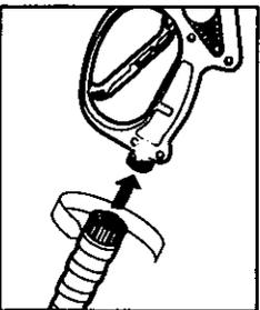
**Step 7** Attach the high pressure hose to the spray gun.
