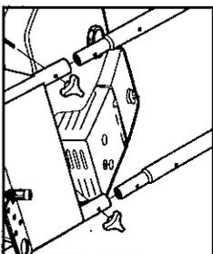
**Step 1** Attach the handle to the frame of the pressure washer. Align pressure washer. Align holes, insert bolts, and tighten with knobs.
