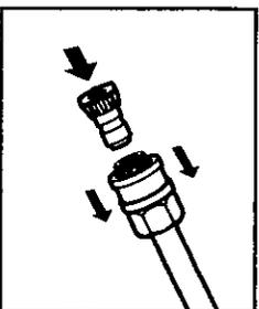
**Step 5** Pull the spring-loaded collar of the wand back to insert your choice of quick connect nozzle.
