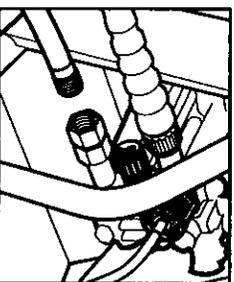
**Step 9** Connect the garden hose to unit's water inlet.
