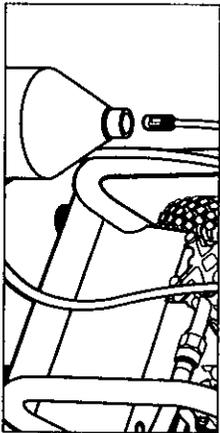
**Step 3** Fill a container with Kärcher detergent. Place the filter end of detergent suction tube into the detergent.
