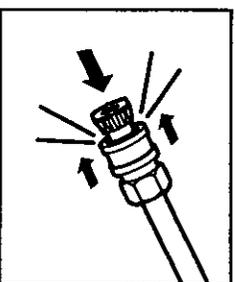
**Step 6** Release the collar and push the nozzle until the collar clicks. Pull the nozzle to make sure it is seated properly.
