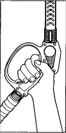
**Step 4** With the engine running, pull trigger to operate unit. Liquid detergent is drawn into the unit and mixed with water. Apply detergent to work area. Do not allow detergent to dry on surface.
