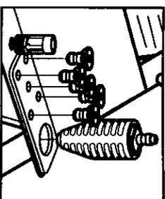
**Step 3** Place the quick connect nozzles in the nozzle holder.
