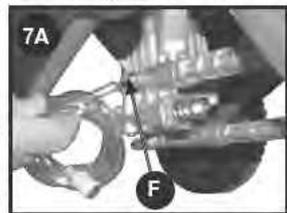
4. After use of chemicals, place detergent siphon hose into container of clean water and draw clean water through chemical injection system to rinse system thoroughly. If chemicals remain in the pump it could be damaged. Pumps damaged due to chemicals will not be covered under warranty.
