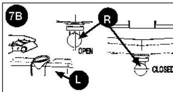
**NOTE:** After use turn valve (R) to CLOSED position.
