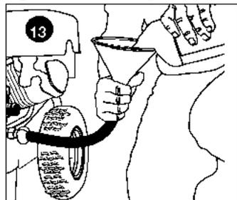
3. Connect the length of garden hose to the water inlet of the pump.
