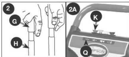
4. Remove the colored quick-connect nozzles (K) from the plastic bag and insert them into correct grommet on the nozzle holder. Nozzles are color coded to match colored nozzles on label (Q).
