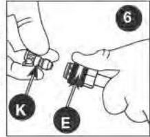
**⚠ WARNING:** Flying object could cause risk of serious injury. Ensure nozzle is completely inserted in quick-connect socket and quick-connect snap ring is fully engaged (forward) before squeezing gun trigger.
