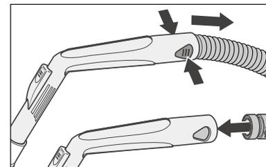
Press in on the left and right hose release clips at the same time to dismantle the hose for cleaning.
