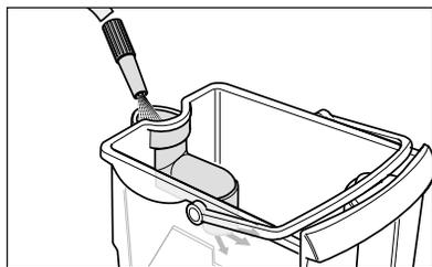
**4. Cleaning the suction manifold in the water filter container**
