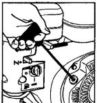
Step 8 Pull the starter handle. If the engine fails to start after 3 pulls, squeeze the trigger gun to release pressure, and repeat step.
