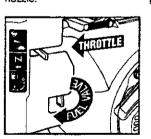
Step 6 Model HD 3101 Slide the fuel valve to the "ON" position. Slide the throttle lever left about 1/3 of the way toward the fast position.
