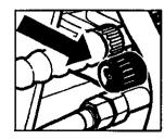
Step 9 Adjust pressure control to desired setting.
