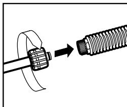
**Step 5** Attach the wand to the spray gun.
