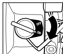
**Step 7** Turn the engine switch to the "ON" position.
