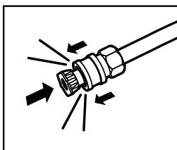
**Step 7** Release the collar and push the nozzle until the collar clicks. Pull the nozzle to make sure it is seated properly.
