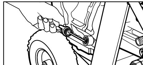
**Step 1** Check oil level. Oil level should be level with the bottom of the oil filler neck. Be sure the machine is level when checking the oil level. (Refer to the engine's operating manual for seasonal grades.) We recommend that the oil be changed after the first 5 hours of use, then once every 50 hours.
