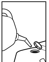
**Step 2** Fill gas tank with unleaded gasoline. Do not use leaded gasoline.
