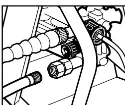
**Step 10** Connect the garden hose to unit's water inlet.
