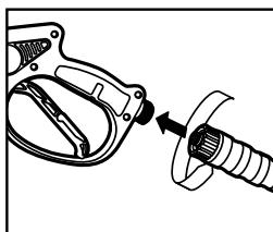
**Step 8** Attach the high pressure hose to the spray gun.
