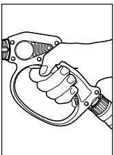
**Step 5** Press trigger to release water pressure.
