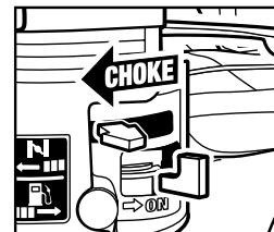
**Step 5** Slide the choke lever to the left to the "CLOSED" position (on a warm engine, leave the choke lever in the open position).
