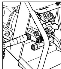
**Step 7** Disconnect high pressure hose from high pressure outlet.
