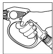
**Step 3** Press trigger to release water pressure.
