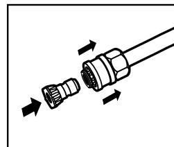
**Step 6** Pull the spring-loaded collar of the wand back to insert your choice of quick connect nozzle.
