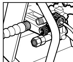
**Step 9** Connect the high pressure hose to the unit's high pressure outlet.
