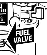
**Step 2** Slide fuel valve to the off position.
