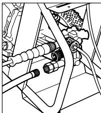
**Step 6** Disconnect garden hose from water inlet on the unit.
