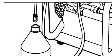
**Step 3** Fill a container with Kärcher detergent. Place the filter end of detergent suction tube into the detergent.
