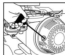
**Step 8** Pull the starter handle. If the engine fails to start after 3 pulls, squeeze the trigger gun to release pressure, and repeat step.
