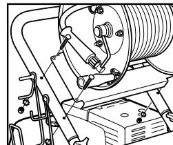
**Step 3** Attach the reel to the handle. Align holes, insert bolts, and tighten with nuts.
