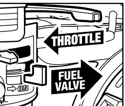
**Step 6** Slide the fuel valve to the "ON" position. Slide the throttle lever left about 1/3 of the way toward the fast position.
