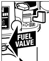
**Step 3** Slide fuel valve to the "OFF" position.
