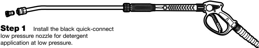
**Step 1** Install the black quick-connect low pressure nozzle for detergent application at low pressure.
