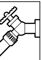
**Step 3** Connect garden hose to the cold water source and turn water on completely. **Never use hot water.**
