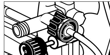
**Step 2** Adjust the dosage control at the beginning of the detergent tube for light (1), or maximum (6) detergent coverage.
