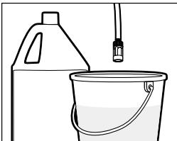
**Step 1** Remove detergent suction tube from container and insert into one gallon of fresh water. Siphon water at low pressure for one minute.
