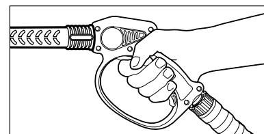
**Step 4** With the engine running, pull trigger to operate unit. Liquid detergent is drawn into the unit and mixed with water. Apply detergent to work area. Do not allow detergent to dry on surface.
