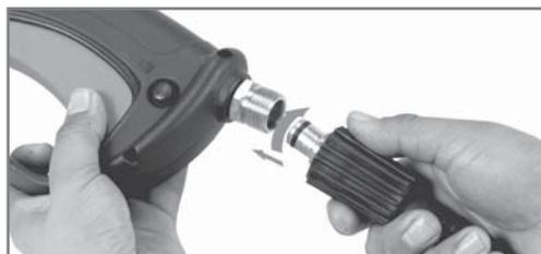
Unpack the pressure hose and connect the metal fitting to the gun inlet. Ensure that the threads are aligned properly and that the connection is secure. Securely tighten the nut by hand. Place the gun into the gun holder on the side of the Pressure Washer.
