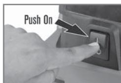
5. Turn on the ON/Off switch on the front of the Pressure Washer. **NOTE:** Motor does not start until trigger is pulled.
