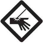
Injection Hazard. The high pressure water jet produced by this tool can cut skin or cause injury to hands or eyes. Do not allow spray to strike you and do not spray toward people or animals. Do not spray the tool itself or any electrical source.
