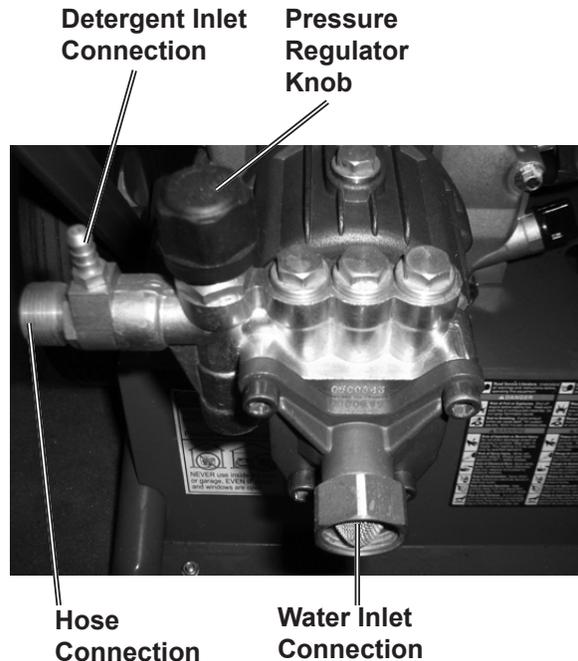
7. Connect the water supply to the Water Inlet Connection. The water source must be able to provide a minimum of five gallons of clean, cold water per minute at 20 PSI. Only use a hose that is rated to meet this capacity.
