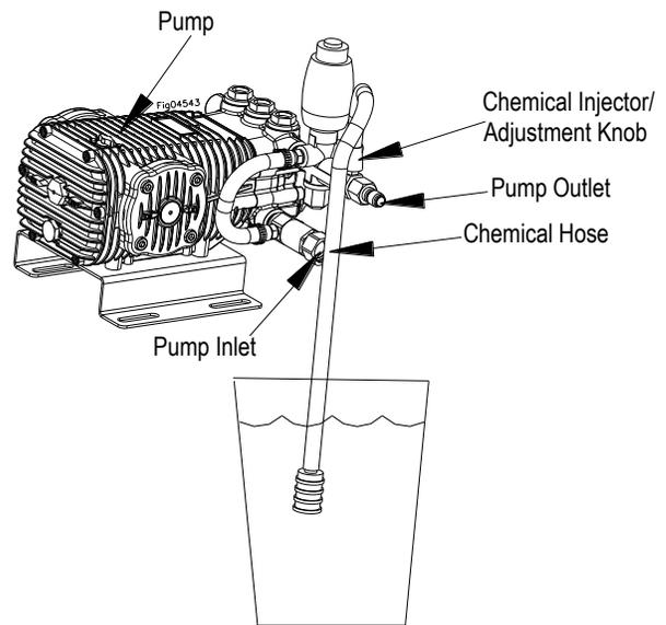
**Note:** Adding accessories (IE: telescoping wands, extra length of High pressure hose, Non factory triggers) will effect chemical injector performance or cause it not to operate at all.
