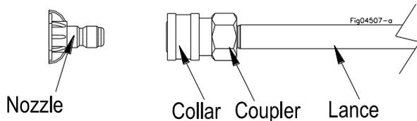
3. Release the collar, making sure it springs back and re-seats to its original (non-retracted) position. Check the connection by pulling on the nozzle to ensure a tight connection -- if correctly inserted, nozzle will rotate but not pull out.
