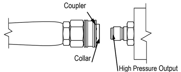
3. Release the collar, making sure it springs back and re-seats to its original (non-retracted) position. *Check the connection by pulling on the hose to ensure a positive connection.*
