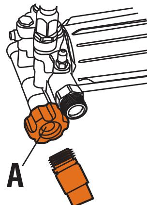
3. Connect the garden hose (not to exceed 50 feet in length) to the water inlet (Figure 12). Tighten by hand.
