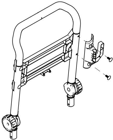
2. Install lance hook to unit frame using (2) supplied tree clips. Align holes and push the tree clips into holes until they sit flush with gun hook (Figure 3).
