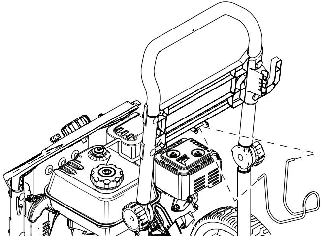
5. Insert color-colored nozzles in spaces provided in front panel (Figure 6).
