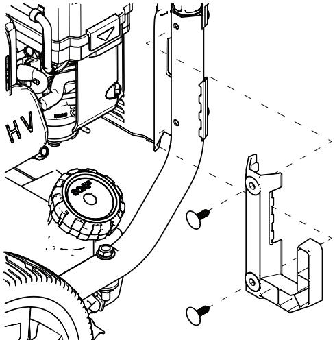
3. Place handle assembly (A) onto cradle supports (B). Allow handle to slide into position. Locate the (4) screws and allen wrench. Install the four screws using supplied allen wrench as shown in (Figure 4).
