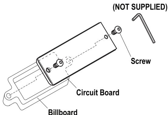
2. Remove the 2 mounting screws.
