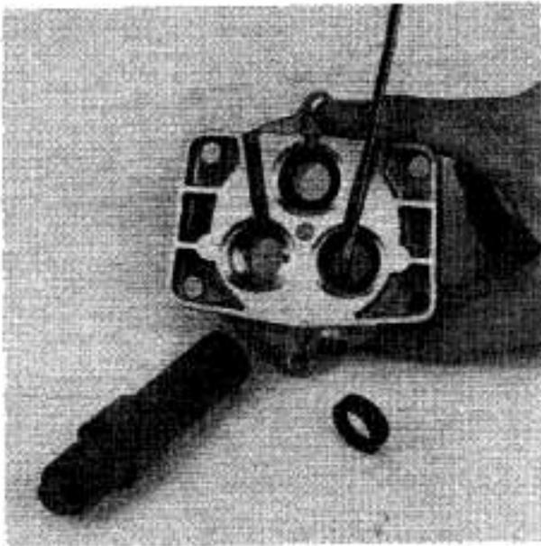
Pass a screwdriver through the leakage grooves and lever out the oil seal rings.
