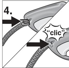
Pull out the locking slide from the right side of the trigger gun handle, and insert the small end of the high pressure hose into place. Push the locking slide back into the trigger gun to lock the hose in position.
