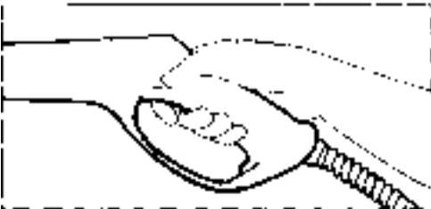
**Step 5** Plug the power cord into the power outlet. Unlock the lock of the trigger gun. Trigger the gun to eliminate trapped air, wait for a steady flow of water to emerge from the spray nozzle.
