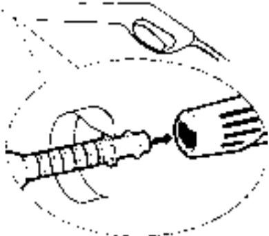
**Step 2** Insert the spray wand of your choice into the trigger gun. Press in against the spring tension and twist into the locked position.
