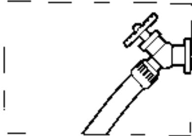
**Step 4** Connect garden hose to the cold water source and turn water on completely.
