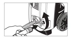
→ STEP 4: Connect garden hose to the cold water source and turn water on completely. Plug the power cord into the power outlet.
