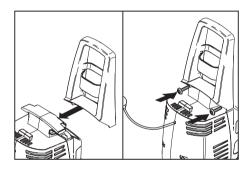
→ STEP 3: Place detergent tank into compartment and attach cap with detergent dosing valve and detergent suction tube.
