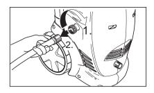
**STEP 5:** Disconnect the high pressure hose from the high pressure outlet.
