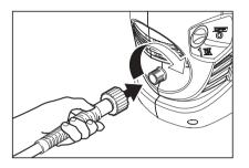
→ STEP 2: Insert the spray wand of your choice to the trigger gun. Press in against the spring tension and twist into locked position.
