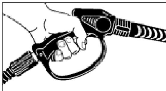
**Step 4** With the engine running, pull trigger to operate unit: Liquid detergent is drawn into the unit and mixed with water. Apply detergent to work area. Do not allow detergent to dry on surface.
