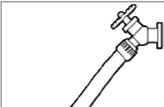
**Step 5** Connect garden hose to the cold water source and turn water on completely.
