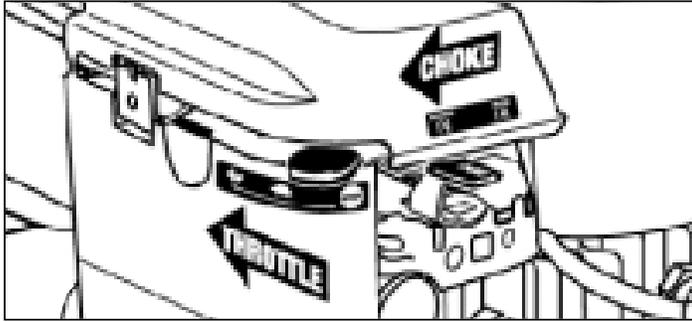
**Step 7** Slide the throttle control to the fast position. Move the choke lever to the “CHOKE” position (only if the engine is cool). After starting, move the choke to “RUN”.
