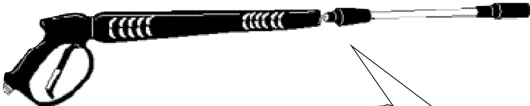
**Step 4** Insert the spray wand into the gun. Push in and turn clockwise to lock spray wand in place. Turn the wand collar clockwise onto the spray wand threads until tight.
