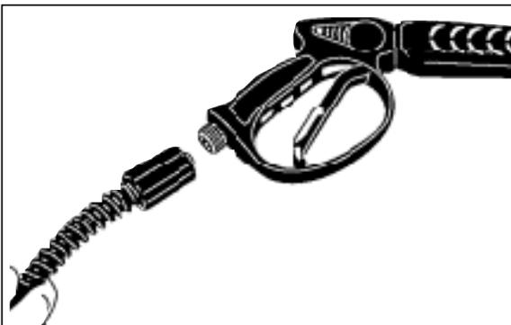
**Step 5** Attach high pressure hose to trigger gun.
