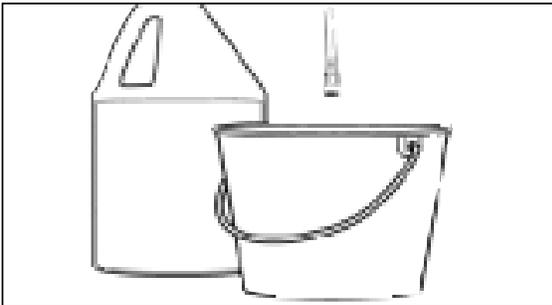
**Step 3** Fill a container with Kärcher detergent. Place the filter end of detergent suction tube into the container. Be sure to adjust the filter by turning it to the desired detergent intake.
