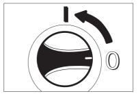
**Step 6**Turn on the pressure washer (I/o<sub>N</sub>).
