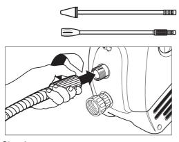
**Step 1**Connect the high pressure hose to the unit's high pressure outlet.
