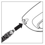
**Step 2** Insert the small end of the high pressure hose into place.
