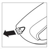
**Step 1**Pull out the locking slide from the right side of the trigger qun handle.
