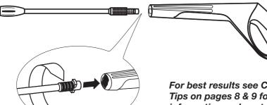
**Step 1** To apply detergents install the Vario spray wand. Set the Vario spray wand to the low pressure setting (-) by turning the wand collar. The wand must be set in the low pressure (-) position to apply detergents.
