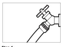
**Step 4**Connect garden hose to the cold water source and turn water on completely.
