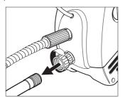
**Step 5**Disconnect the garden hose from the water inlet on the unit.
