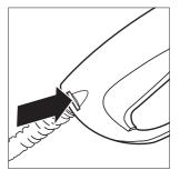
**Step 3**Push the locking slide back into the trigger gun to lock the hose in position.
