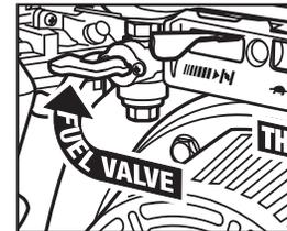
**Step 6** Turn the fuel valve to the "ON" position. Slide the throttle lever left about 1/3 of the way toward the fast position.
