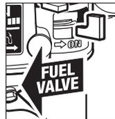
**Step 2** Slide fuel valve to the off position.
