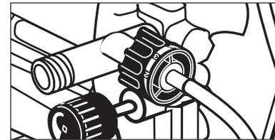
**Step 2** Adjust the dosage control at the beginning of the detergent tube for light (1), or maximum (6) detergent coverage.
