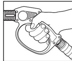
**Step 4** Trigger the gun to eliminate trapped air, wait for a steady flow of water to emerge from the spray nozzle.
