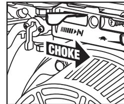
**Step 5** Slide the choke lever to the "CLOSED" position (on a warm engine, leave the choke lever in the open position).
