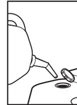
**Step 2** Fill gas tank with unleaded gasoline. Do not use leaded gasoline.
