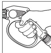
**Step 3** Press trigger to release water pressure.
