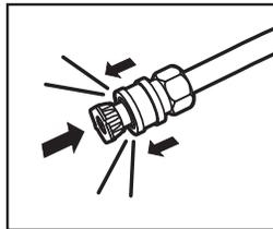
**Step 6** Release the collar and push the nozzle until the collar clicks. Pull the nozzle to make sure it is seated properly.
