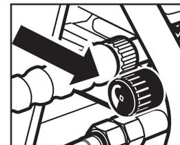
**Step 9** Adjust pressure control to desired setting.
