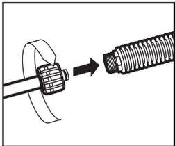
**3** **Step 4** Attach the wand to the spray gun.
