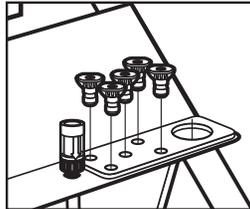
**Step 3** Place the quick connect nozzles in the nozzle holder.
