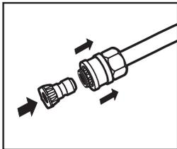
**Step 5** Pull the spring-loaded collar of the wand back to insert your choice of quick connect nozzle.
