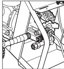
**Step 7** Disconnect high pressure hose from high pressure outlet.
