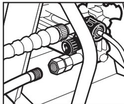
**Step 9** Connect the garden hose to unit's water inlet.
