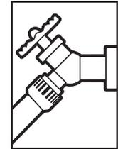
**Step 3** Connect garden hose to the cold water source and turn water on completely.
