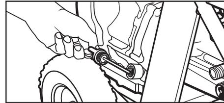
**Step 1** Check oil level. Oil level should be level with the bottom of the oil filler neck. Be sure the machine is level when checking the oil level. (Refer to the engine's operating manual for seasonal grades.)
