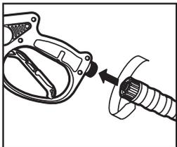
**Step 7** Attach the high pressure hose to the spray gun.
