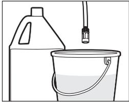
**Step 1** Remove detergent suction tube from container and insert into one gallon of fresh water. Siphon water at low pressure for one minute.
