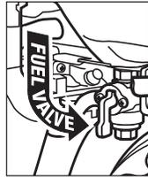
**Step 3** Turn fuel valve to the "OFF" position.
