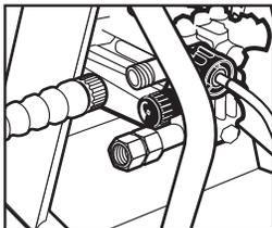
**Step 8** Connect the high pressure hose to the unit's high pressure outlet.
