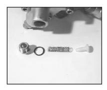
2. Remove the valve spring (18) and valve cone (36) from the manifold (35). Inspect the parts for wear and replace as necessary.
