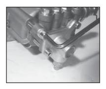
8. Next, remove the four manifold bolts (40) with a 6mm allen wrench.
