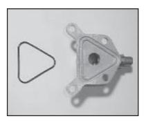
9. Remove the suction flange (39) and flange o-ring (38). Inspect the o-ring for wear and replace as necessary.
