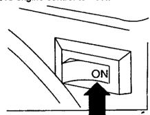
• Turn fuel shut-off valve to "ON" position.
