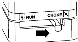
Note: If restarting a warm engine after a short shutdown, move choke lever to "RUN."
