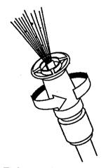
Twist nozzle counterclockwise for "fan" pattern.
