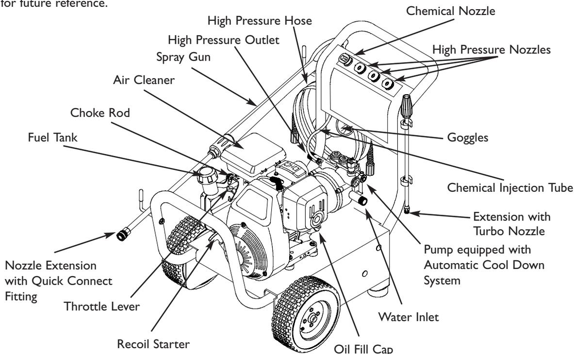
**Air Cleaner** — Dry type filter element limits the amount of dirt and dust that gets in the engine.
