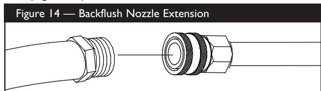
6. Reinstall the nozzle and in-line filter into the nozzle extension.
