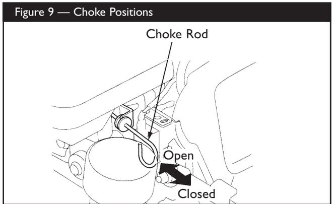
**NOTE:** For a warm engine, be sure the choke is in the **OPEN** position (no choke).
