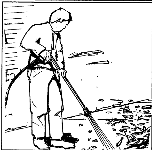
Figure 17 — Testing the Spray Pattern
